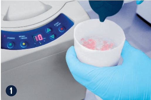
1 Measure out the amount of alginate powder and water and place in the mixing cup.
