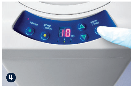
4 Close the Cavex Alginate Mixer and press start.
