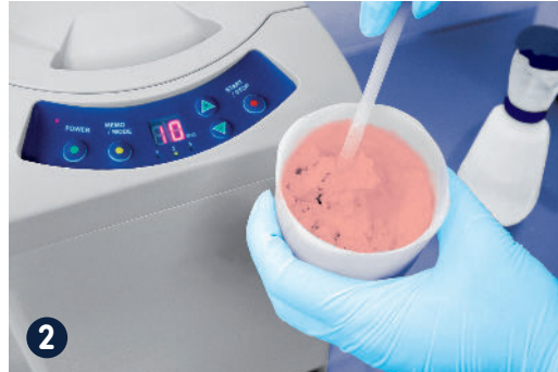
2 Always stir first! This makes cleaning easier and helps keep the appliance in proper working order.
